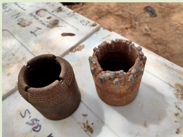
Figure 4. Drilling process and drilling bit from Lakhpat Punrajpur mine 11
